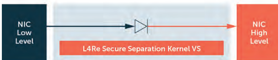
Functional Principle of a Data Diode
